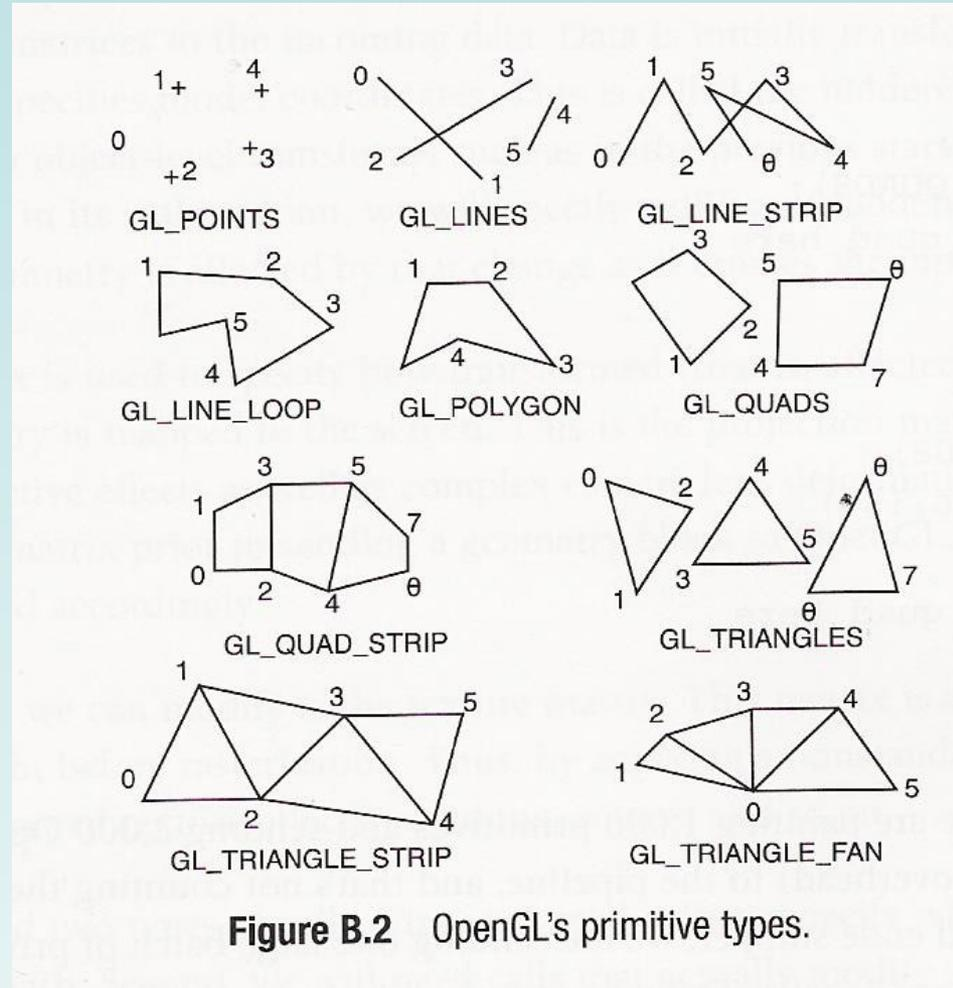
**Figure B.2** OpenGL's primitive types.
